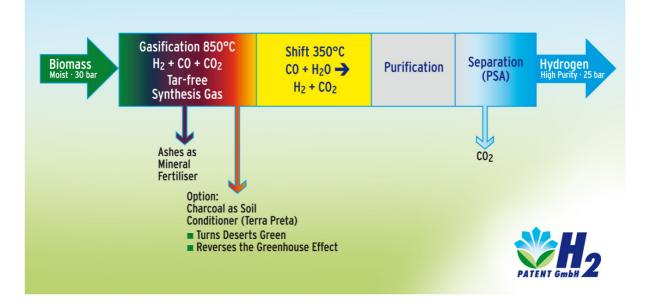
In order to produce pure hydrogen (99,999%), H<sub>2</sub>-Patent GmbH chose pressurised, cascaded fluidised bed reactors to gasify the biomass. This has the following advantages:
